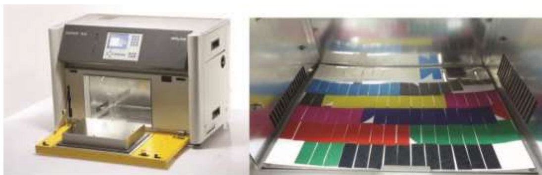
Fig. 1. Treatment of printed substrates in a SUNTEST XSL+ test chamber
