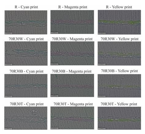
**Figure 1.** Microscopic cross-sectional images of printed paper substrates (R, 70R30W, 70R30B, and 70R30T) in epoxy resin at  $200 \times$  magnification.
