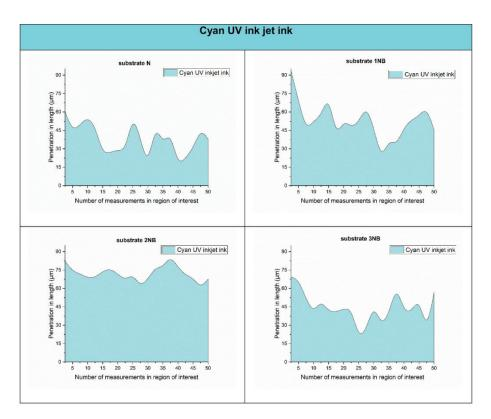
Figure 4. Penetration profile of cyan ink into laboratory substrates
